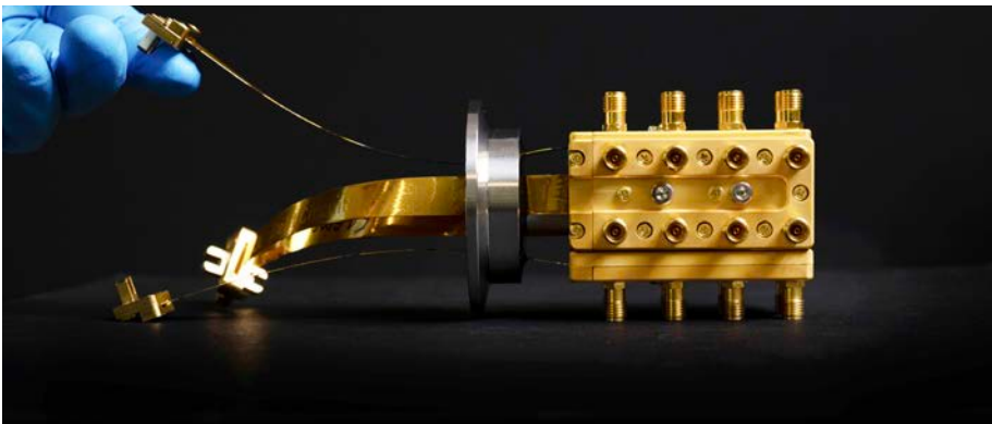
These vacuum ports are available as standard on typical dilution refrigerators and are usually used for readout lines or other important peripherals. The main ports where the I/O modules are entered are typically used for control I/O lines. (Source: Delft Circuits)
