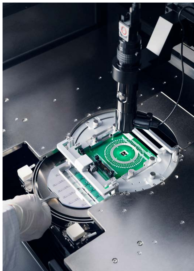
Wafer probe station in the SemiQon lab (Source: SemiQon)
